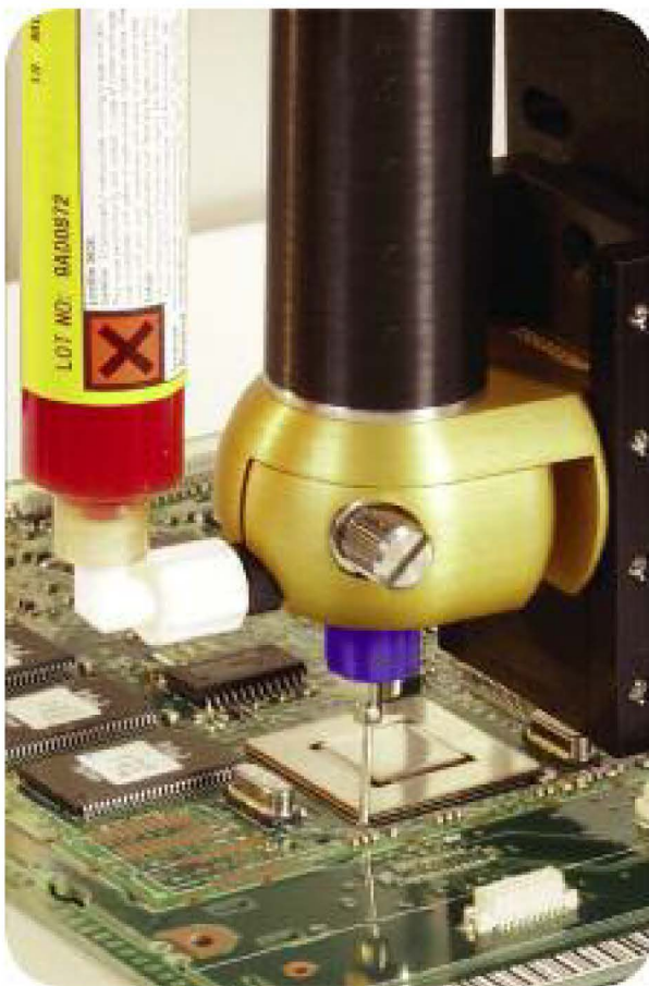
TS5000DMP - performing underfill.
