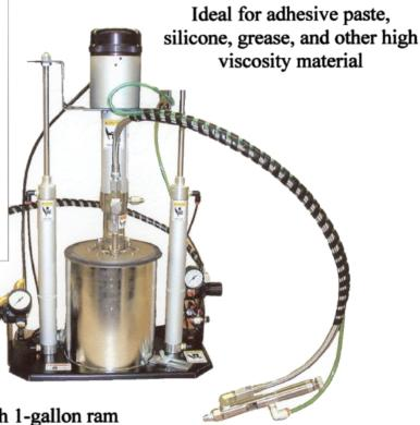
System shown with 1-gallon ram pump, AC992 timing console, and MV 0180 mini valve.
