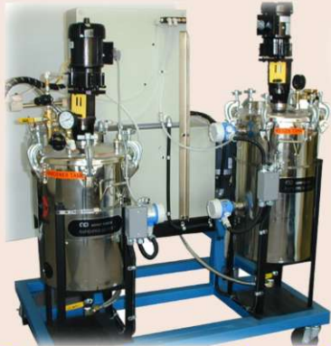
Vacuum degas tanks with agitation and Hi/Low level sensors
