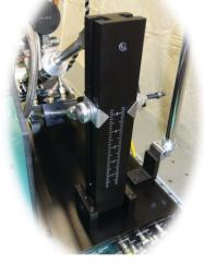
Ratio may be adjusted using the graduated metering cylinder lever arm.
